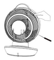
2. Squeeze the two tabs to the left and right of the screws and pull away. At the front of the fan blades there is a locking cap – unscrew the cap in a clockwise motion to remove the fan blades.
