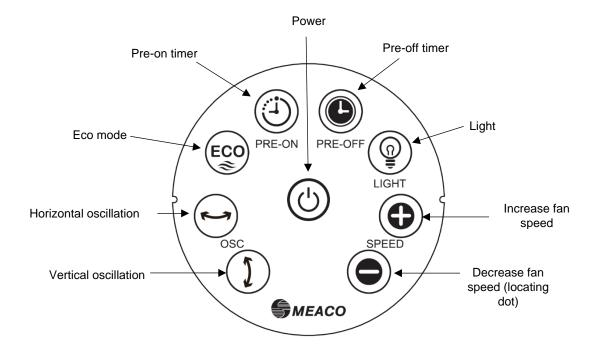
The following functions are only available via the remote control. All other buttons on the remote-control work in the same way as the control panel (see page 4). The remote control has a range of approximately three metres. Before using the remote control, remove the plastic tab.
