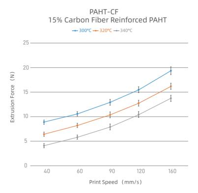
Test parameters: 12mm length brass heat block, BMG extruder, Phaetus Hardened Steel Nozzle, Nozzle size 0.4mm, Layer Height 0.2mm.
