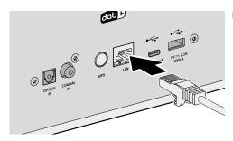
► Connect the LAN cable with the device.
