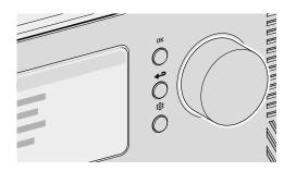
The device is controlled and operation using the navigation keys and the control (e.g. to select menu item the instructions on the display). The device is controlled and operated using the navigation keys and the rotary control (e.g. to select menu items or follow
