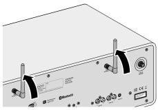
▶ Point the antennas upwards.
