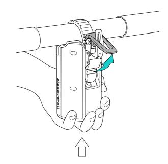
**4.** Keep the product **vertical** as you tighten the ratchett. Tighten by rotating the ratchett lever (marked in grey) upwards, repeating until tight. The product should be firmly attached (not loose), but do not tighten so much that it deforms the product or stroller.
