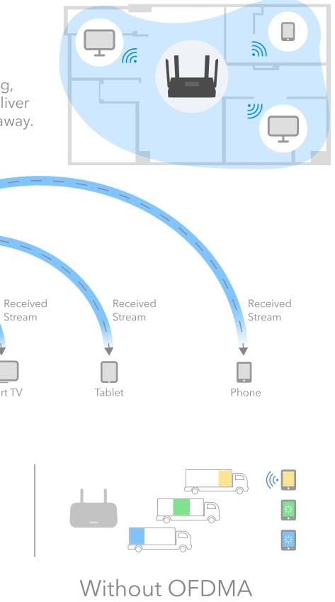
More Devices: Wi-Fi 6 uses OFDMA to improve capacity and efficiency of your network, so more devices can connect without slowing down your Wi-Fi.
