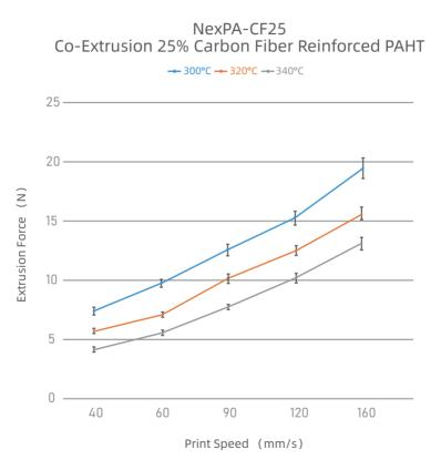
Test parameters: 12mm length brass heat block, BMG extruder, Phaetus Hardened Steel Nozzle, Nozzle size 0.4mm, Layer Height 0.2mm.
