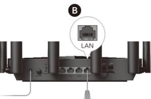
**B Wired:** Turn off the Wi-Fi on your device and connect it to the router's LAN port via an Ethernet cable.
